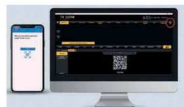
FIGURE 15 Linking the app to the patient database via a QR code generated by clicking on screen (the icon in the red circle)
