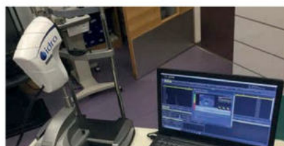
FIGURE 1 The IDRA fits to a slit-lamp base and links to software in a laptop
