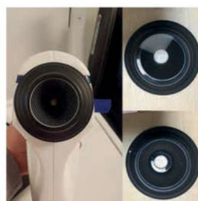
FIGURE 3 Two adaptor heads can be fitted. A wedge target (top right) for interferometry and a Placido-style (bottom right) for surface profile assessments
