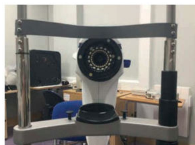
FIGURE 2 The LED lights on the base unit. Note the blue tab for insertion of an orange absorption filter for blue light assessment
